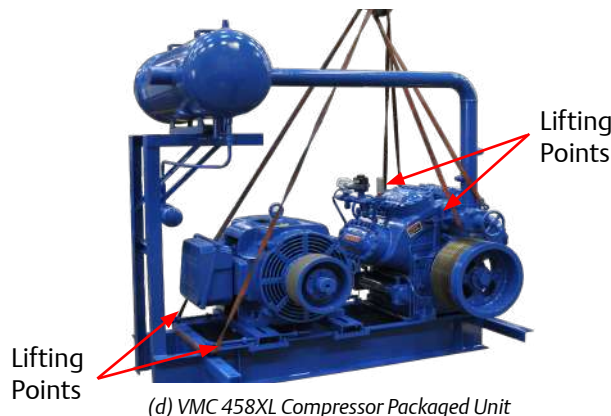
Figure 3-1. Rigging and Lifting Points
