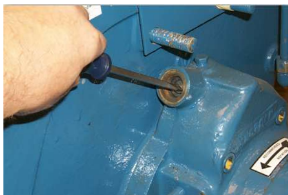
Figure 4-2. Oil Pressure Regulating Valve Adjustment
